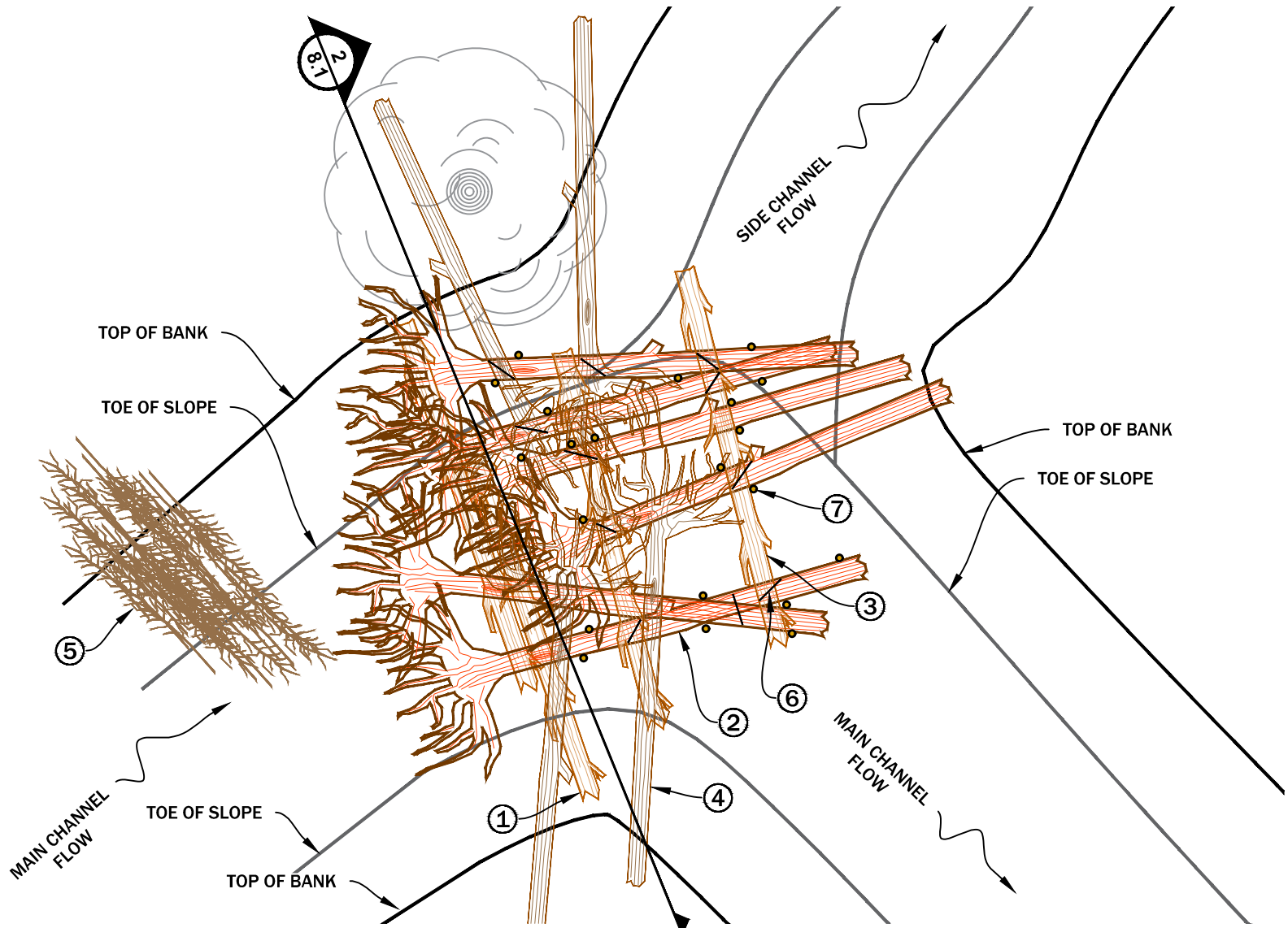
1 HELICOPTER PLACED LARGE WOOD APEX PLAN VIEW 1" = 12'
